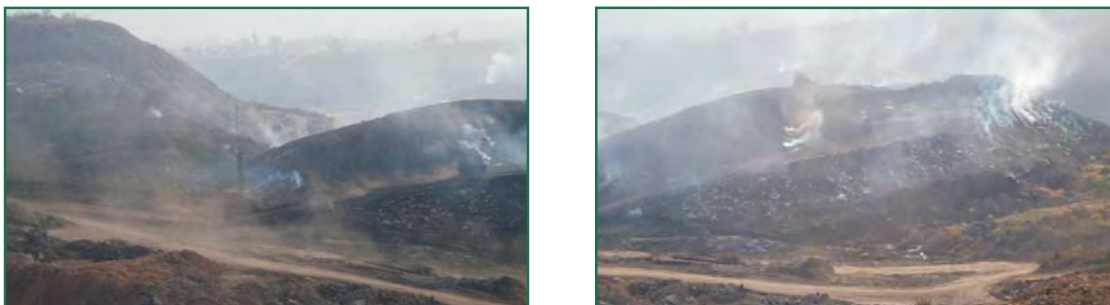
Fig. 1 - Fugitive emissions of particulate matter and gases during coal mining
